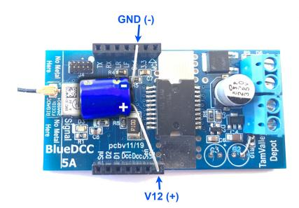
When running the 5 amp board on AC Trackpower using a Lionel power pack that outputs "chopped sine wave", add a 35 volt (or higher) 470 microfarad electrolytic capacitor as shown.
